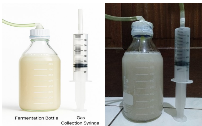
Figure 2. The Enrichment Process of the Mixed EAB Culture Lasted for 20 Days; (a) Schematic and (b) Photograph of the Enrichment System
